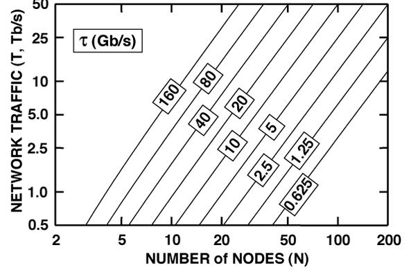
Fig. 4. Traffic demand bit rate. The traffic demand bit rate  $\tau(N, T)$  for uniform demand is graphed as a function of the number of nodes  $N$  and total two-way traffic  $T$  using a contour plot. Contours of constant  $\tau$  are labeled in units of gigabits per second.
