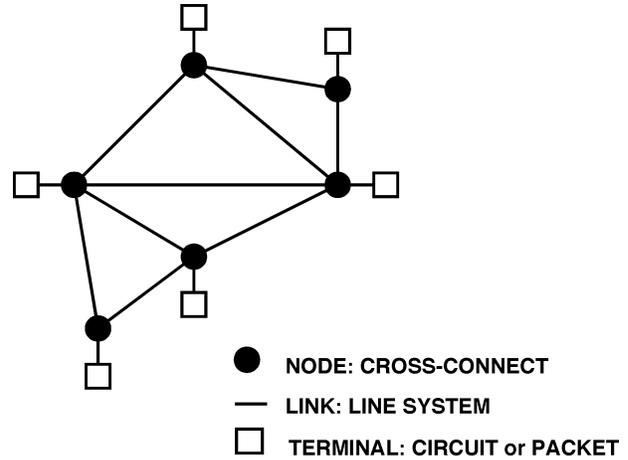
Fig. 1. Mesh network architecture. The average degree of node is  $\langle \delta \rangle = 3$  for this network topology of  $N = 6$  nodes and  $L = 9$  links.
