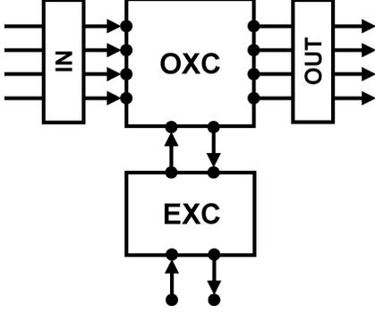
Fig. 8. Bandwidth management architecture using both OXCs and EXCs. For a cross connect using only electronic bandwidth management, a single EXC replaces the combination of OXC and EXC.
