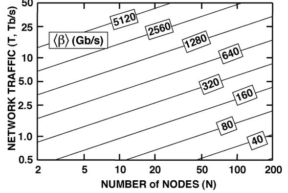
Fig. 5. Mean traffic on link. The mean traffic on a link  $\langle \beta^k(N, T) \rangle$  for uniform demand with restoration is graphed as a function of the number of nodes  $N$  and total two-way traffic  $T$  under the constraint  $\langle \delta \rangle = 3.5$  using a contour plot.
