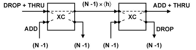
Fig. 6. Demands and cross-connect ports. The figure serves as a guide to count the number of cross-connect ports occupied by a demand as it traverses the network. The relationship among the local add, drop, and through channels is also depicted. Here, the numbers of add and drop demands, each  $N - 1$ , specifically correspond to the uniform demand model.
