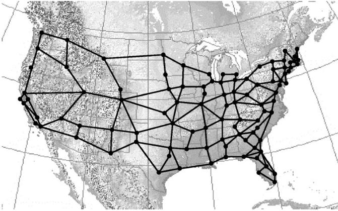
Fig. 2. Prototypical backbone network. Illustrated is a hypothetical core fiber transport network indicative of the larger inter-exchange carriers of the continental United States. This example network consists of 100 nodes and 171 links [6]. The average degree of nodes is  $\langle \delta \rangle = 3.4$ , and the average number of minimum hops between node pairs is  $\langle h \rangle = 6.6$ . (Background relief map courtesy of the U.S. Department of the Interior.)
