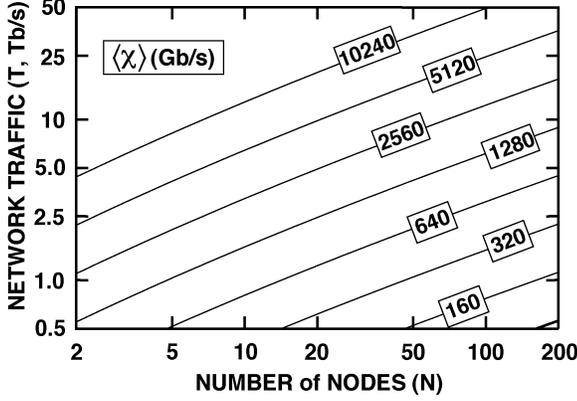
Fig. 7. Mean cross-connect traffic. The mean traffic entering a cross-connect  $\langle \chi^\kappa(N, T) \rangle$  for uniform demand with restoration is graphed as a function of the number of nodes  $N$  and total two-way traffic  $T$  under the constraint  $\langle \delta \rangle = 3.5$  using a contour plot.
